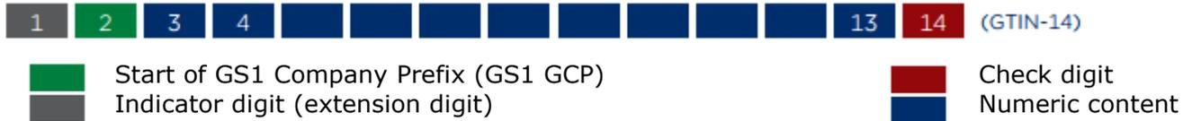
If you are using SGTIN, AI (Application Identifier) 21 is used to register the serial number. This is explained in chapter 4.1. Serial number cannot exceed 20 digits / alphanumeric characters
