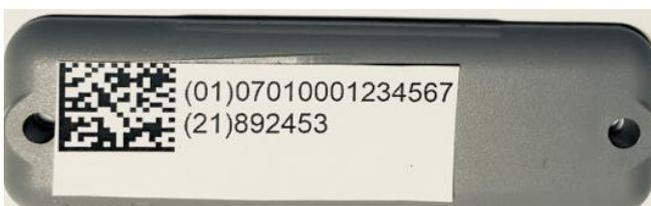
\* This RFID tag has a label with a GS1 Datamatrix 2D barcode attached to it.
